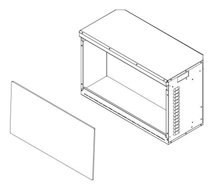
3. Unscrew the screws located on each side and take off the inner side steel panels.
